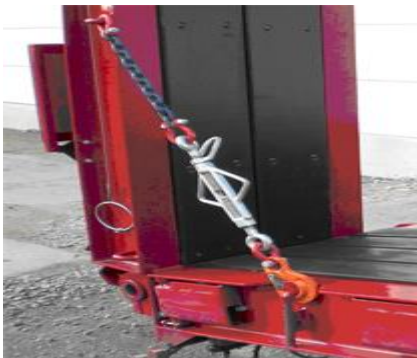
Photograph 3: Turnbuckle tensioning device with lock nut
