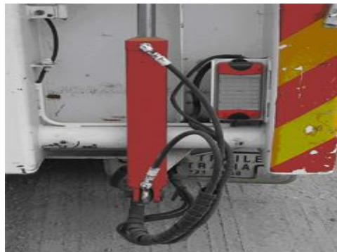
Photograph 4: Double acting hydraulic cylinder (note: two hydraulic lines)
